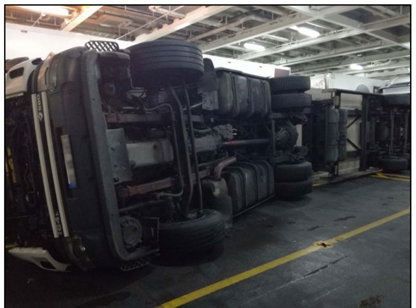
Figure 3: Truck toppled over on main deck
