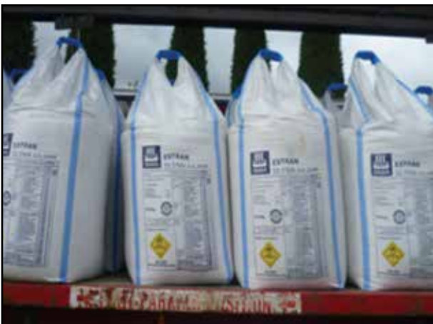
Not secured in a curtainsider – unacceptable.
